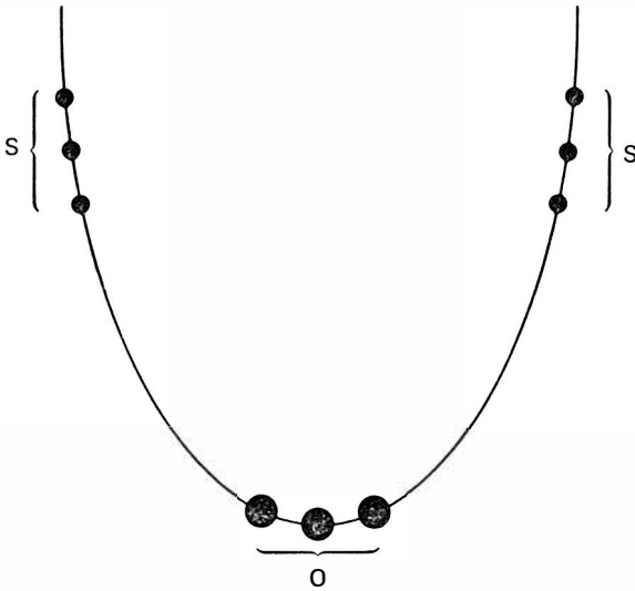
Figure 2. String or cord with knotted SOS message in Morse Code. Three smaller knots represent the Morse Code dots = "S" and the three bigger knots represent the Morse Code dashes = "O".
