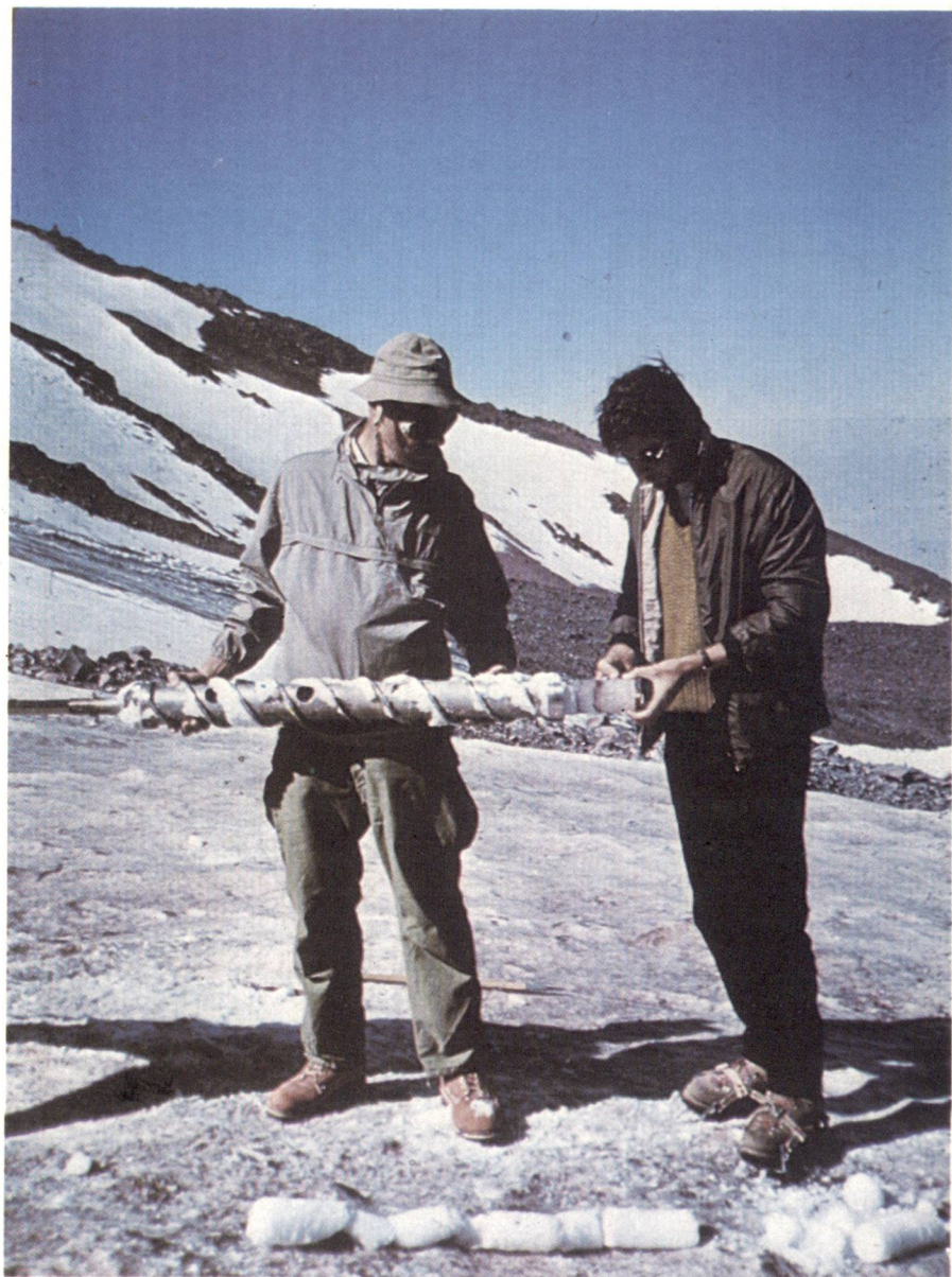
The SEARCH boring efforts through the ice pack were unsuccessful because the bit frequently hit rocks and became permanently damaged. Two SEARCH team members survey the bit damage just after boring.
